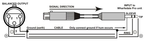
UNBALANCED INPUT AND OUTPUT WIRING WITH MONO 1/4" JACK CONNECTIONS
